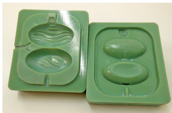
A 3D printed injection mold for a Domestos-brand toilet rim block
